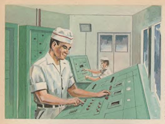
The automatic control equipment belongs to an analogue computer for the world's first fully automatic system for making ice cream mix. It calculates ice cream formulae and converts the information to coded punch cards. These in turn are translated through a batch-blending system to direct the flow of raw products from storage to blending tanks. Wouldn't it be a shame if the "robot" would develop a taste for ice cream and eat it up before it reaches you?
